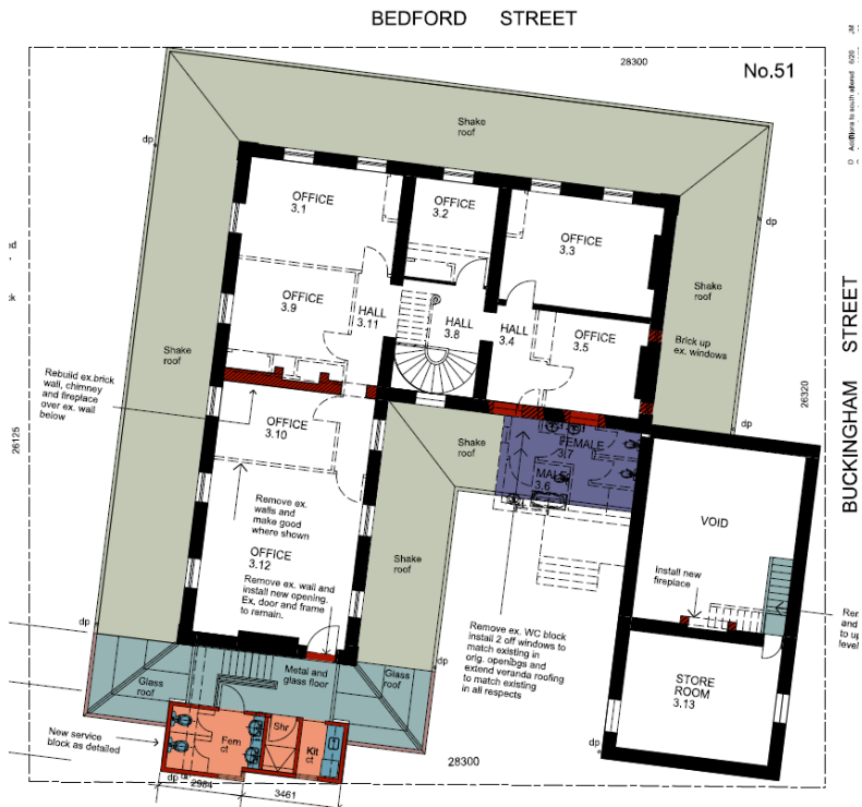
Figure 10: Proposed first floor plan
